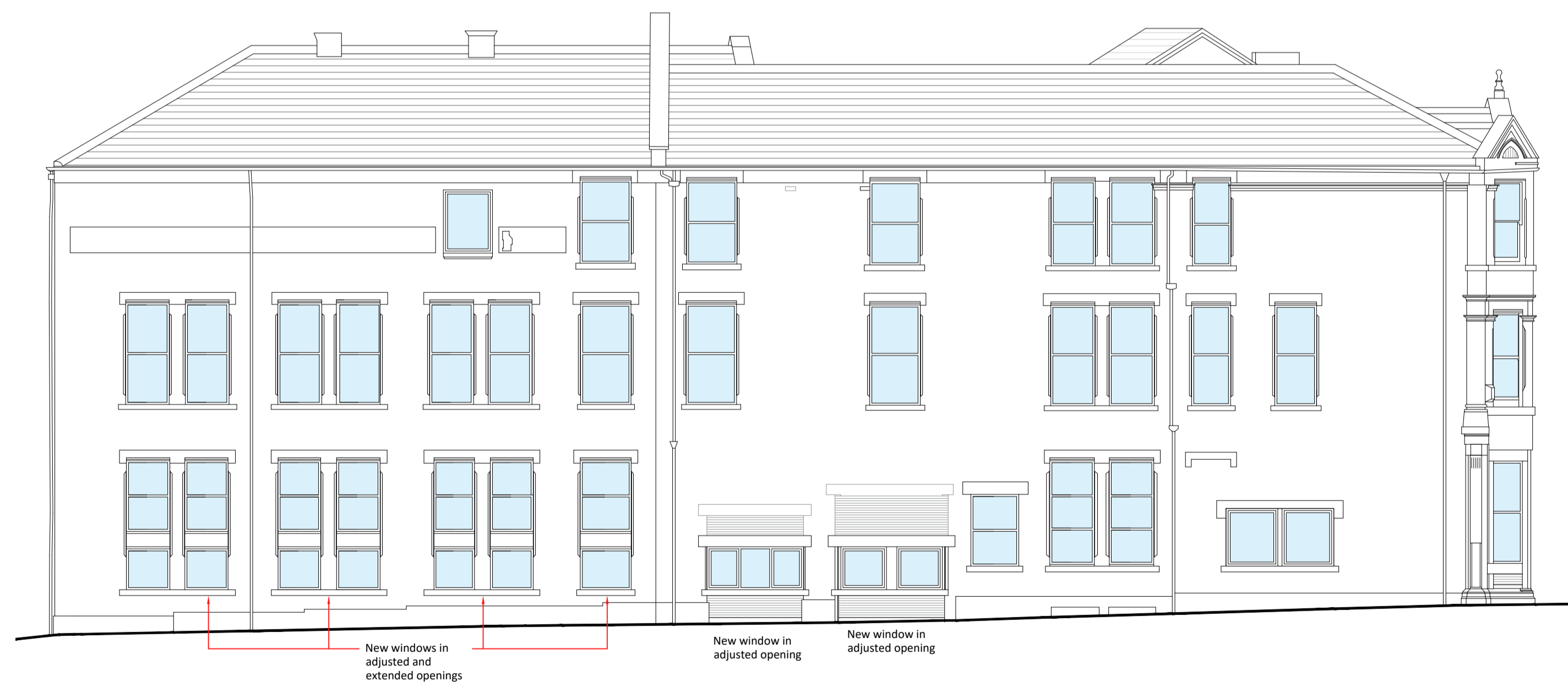
Gable Elevation as Proposed Scale @ 1 : 100
